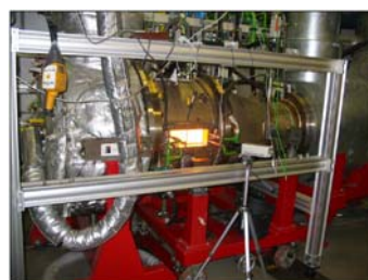
Atmospheric test rig arrangement (SIEMENS burner)
